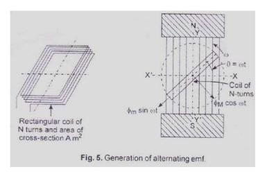
If the coil rotates at an angular velocity of  $\omega$  radians per second then after a time of t seconds the coil will make an angle of  $\theta$ =  $\omega$ t degrees with the horizontal i.e. starting position.
