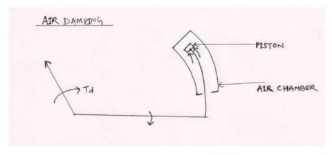
Figure: 7.1(g) Air friction damping
