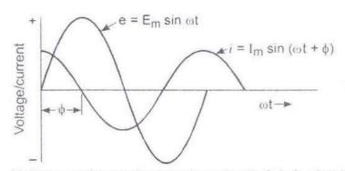
Voltage, and current waves in series R-C A.C. circuit.
