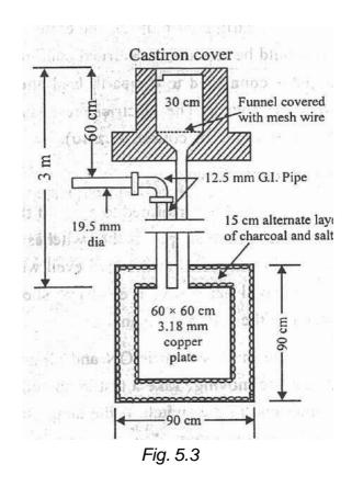
After placing the plate at the bottom of the pit, it is covered with nearly 15cm thick alternate layers of salt and charcoal. Then the bolted earth wire is drawn through GI pipe to the body of the mainswitch.
