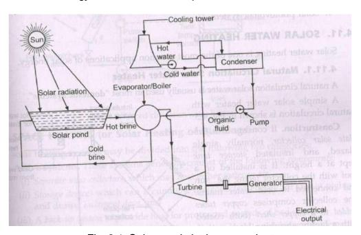
Fig. 8.1. Solar pond elctric power plant
