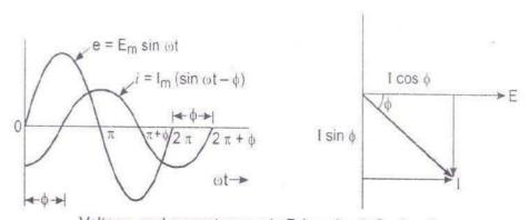
Voltage, and current waves in R-L series A.C. circuit.
