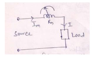
Fig.7.7(a) PMMC with low current
