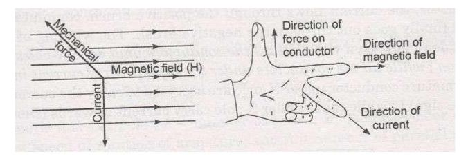
Direction of force experienced on a conductor carrying current, when placed in a magnetic field is given by Fleming's left-hand rule.
