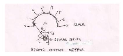
Figure 7.3.1(b) Spring Control Method
