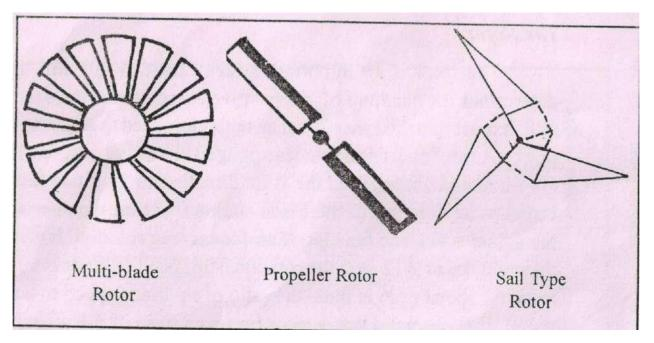
Fig.8.4 Wind mill rotors
