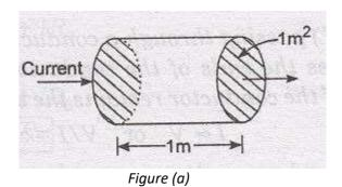
[In the figure(a) above a conductor is shown with its length(L) = 1 metre & Area of cross-section(A) =  $1m^2$ ]
