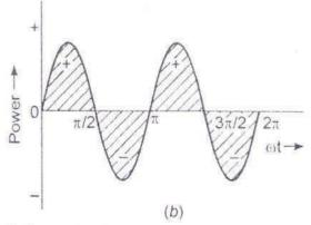
Graphs for A.C. circuit containing inductance only for: (a) voltage, and current; (b) power
