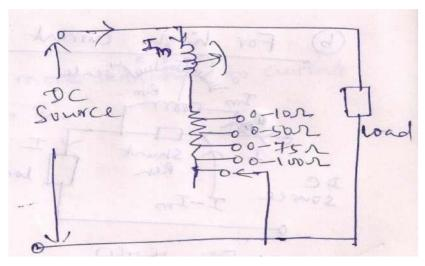
Fig.7.7(e)PMMC as Voltmeter(Multiple range)
