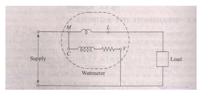
Fig. 7.5.2(a) Circuit diagram of a dynamometer type wattmeter.
