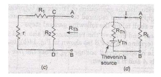
Step III: Remove the voltage source from the circuit, leaving behind only its internal resistance(r) as shown in Figure (c) above. Now, view the circuit inwards .It is found that the circuit now consists of two parallel paths i.e. one containing resistance  $R_2$  only and the other containing resistances  $R_1$ & r in series. Consequently the equivalent circuit resistance( $R_{TH}$ ) as viewed from open circuit terminals A and B is given by:
