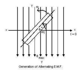
Suppose the flux of a coil having N turns, changes from initial value  $\varphi_1$  weber to the final value of  $\varphi_2$  weber in t seconds. Then , the initial flux linkage = [No. of Turns] x [initial flux linked with coil] =  $N \varphi_1$
