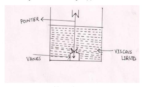
Figure: 7.1(h) Fluid friction damping
