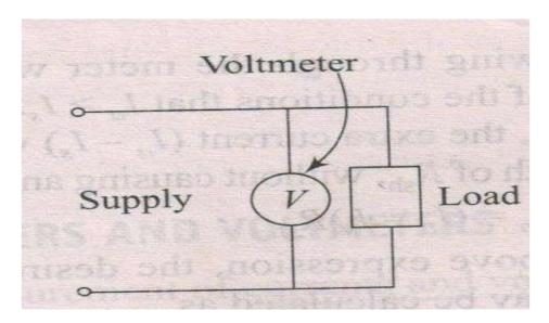
Fig. 7.5.4. Circuit diagram for voltmeter
