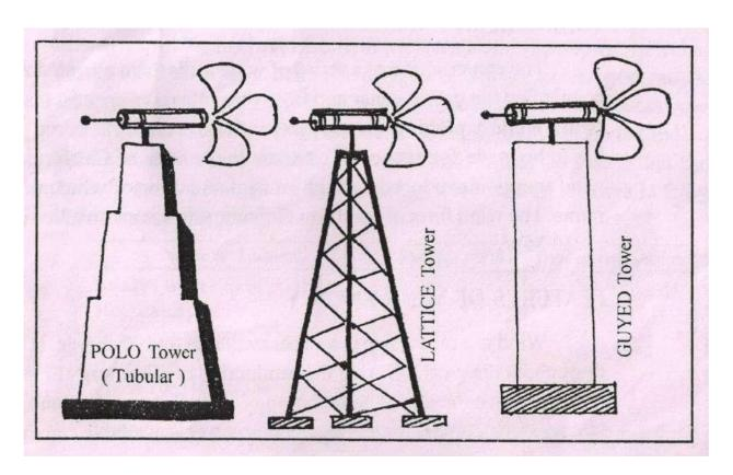
Fig.8.3Wind mill Towers
