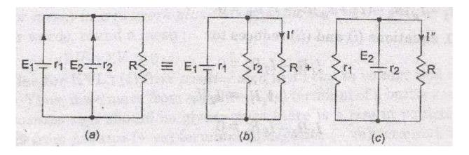
[ Figure(a) with the circuit with two Sources( $E_1\&E_2$ )]
