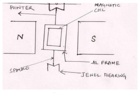
Figure: 7.1(f) Eddy-current damping
