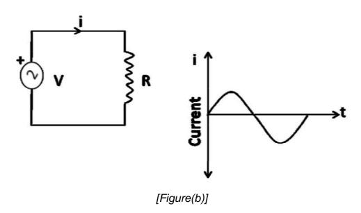
The AC current shown in the above circuit reverses it direction after some time as you see in the wave form diagram.
