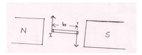
Fig. 7.3(c) Arrangement of conductor inside magnetic field
