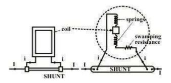
Fig.7.4 Multi-range ammeter circuit.
