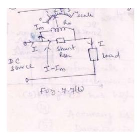
Fig.7.7(b)PMMC with high current rating
