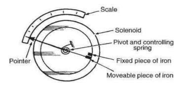
Fig.7.10 Repulsion type instrument.
