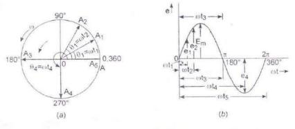
Fig. 7. Phasor (or vector) representation of alternating emf
