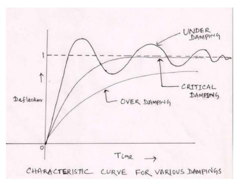
Figure: 7.1(e)Damping Characteristics
