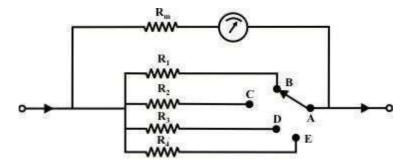
Fig. 7.5(a) Multi-range ammeter circuit.
