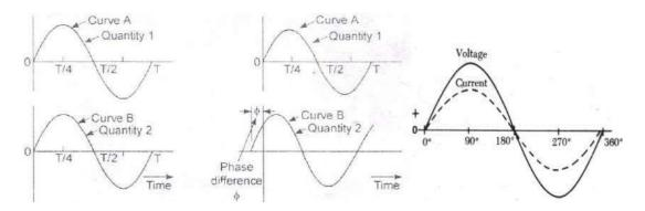
INSTANTANEOUS VALUE: The value of an alternating quantity at any instant is called its instantaneous value.
