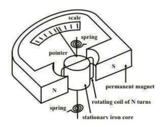
Figure 7.3(a) PermanentMagnet Magnet Moving Coil Instrument.
