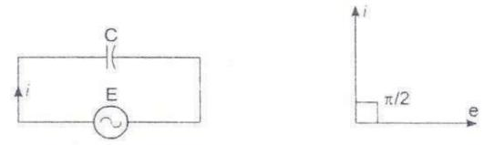
A.C. through purely capacitive circuit
