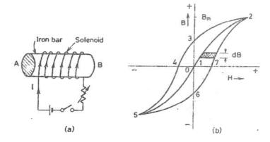
Now if value of H is decreased slowly (by decreasing the current in the solenoid) the corresponding value of flux density (B) does not decreases along 2-1 but decreases some what less rapidly along 2 to 3. Consequently during the reversal of magnetization, the value of B is not zero, but is '13' at H=
