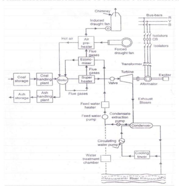
Working of Thermal power Plant: When the water from condenser is fed to the Boiler through Economiser it remains a little hot. The Boiler is a extremely heated chamber because of acontinuous burning of Coal in presence of air injected by F.D fan throughpre-heater.
