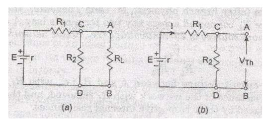
Step I : Disconnect & remove the resistance of the load resistance( $R_L$ ) under consideration from the terminals A & B to get open circuit.
