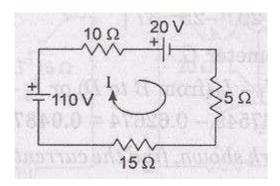
Solution: Applying Kirchoff's voltage Law to the circuit shown above and assuming the current direction to be as shown let us move in the direction of current and write down the equations.
