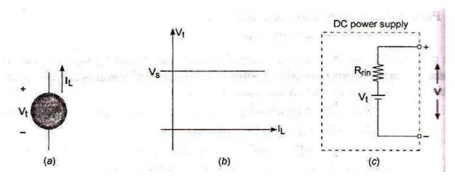
(Figure (a) shows symbol of Ideal voltage source), (Figure (b) shows plot of  $V_tVs$   $I_Lof$  an Ideal voltage source), Figure (c) shows a practical voltage source)
